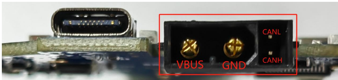
Board terminal model XT30PB(2+2)-M, wire end model XT30(2+2)-F, brand manufacturer AMASS.
